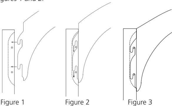
The corner of the arch will be level with the top of the upright and both pins engaged when it is correctly attached. See figure 3.
