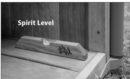
Levelling Tip: The bubble in the level indicates if your unit is sloping. The bubble will always slide toward the highest point, so add height to the opposite corner until the bubble comes to rest in the centre of the glass, between the two lines.
