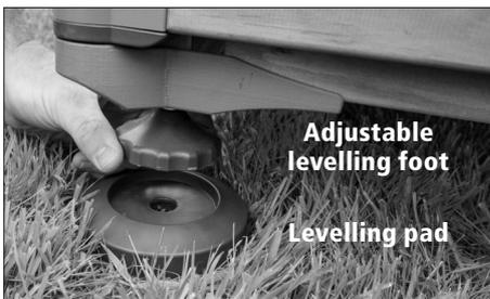
3. Using a spirit level, check to make sure the Unit is not sloped in any direction. Check both side-to-side and front-to-back.
